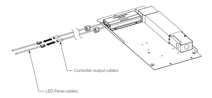
**Tunable White (TNW) Luminaires:** LED Panel cables plug directly into controller. Use controller outputs 1 and 3 for TNW luminaires.
