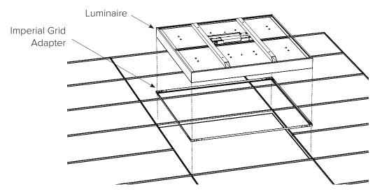
CAUTION: Weight of one FABRILum luminaire is 14kg/31 lbs. The Imperial Grid Adapter required for inch-sized (imperial) ceiling grid weighs an additional 0.8kg/1.75lbs.
